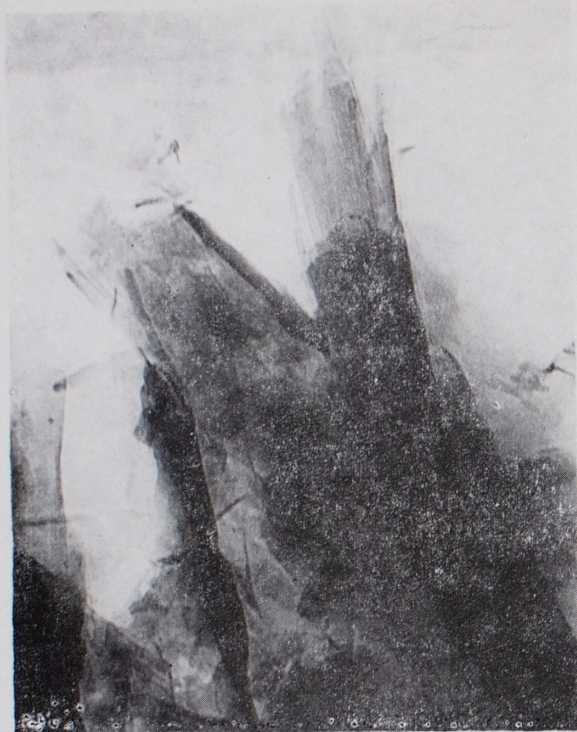
Phot. 3. Sepiolite. Forms of flat laths tangled at the ends and folded at the edges. Magn. \times 100\ 000
