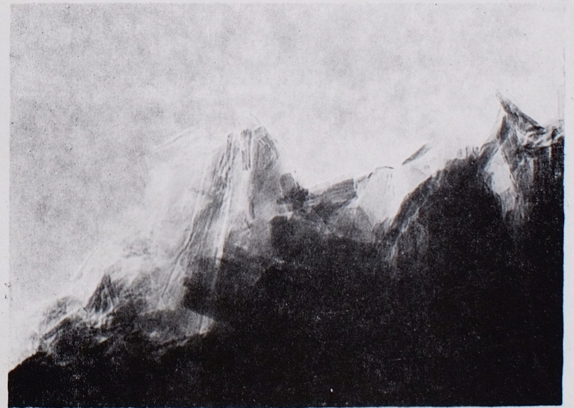
Phot. 2. Sepiolite. Larger aggregate of plates and flakes with irregular shape. Magn. \times 66\ 000
