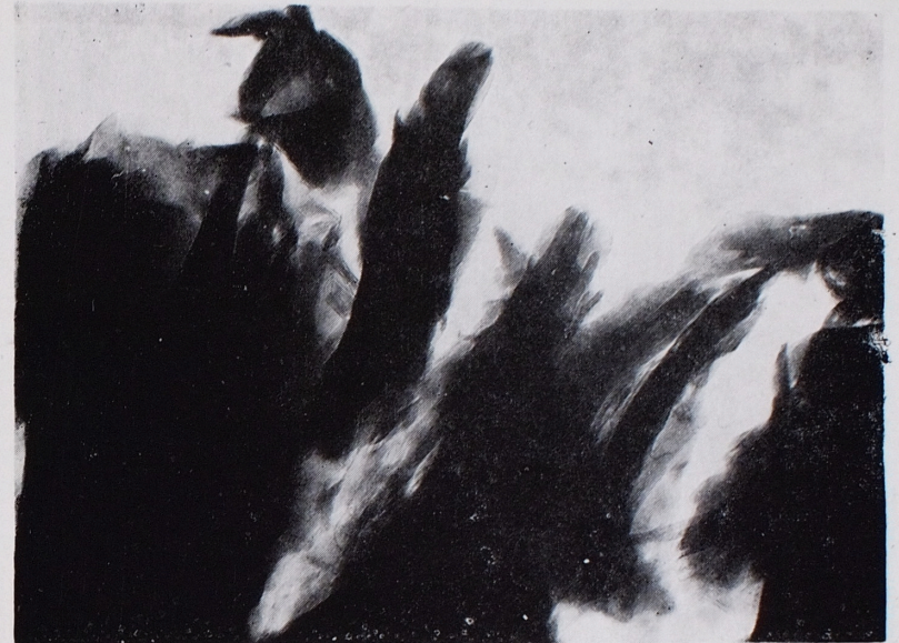
Phot. 1. Sepiolite crystals exhibit a lath-flaky structure. Magn. \times 66\ 000
