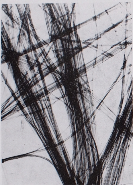
Phot. 7. Hair-like structure of palygorskite. Width of single fibres varies from 500 to 200 Å. They are grouped in parallel branching off ribbons. Magn. \times 32\ 000
